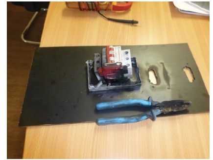
Arc marks on the pliers held by the victim
