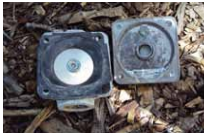
Water damaged regulator
