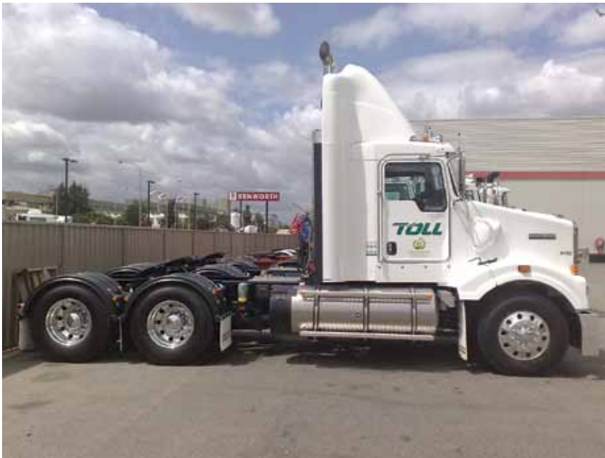
View of Kenworth truck with Westport HPDI system showing one of two multiple LNG containers.
