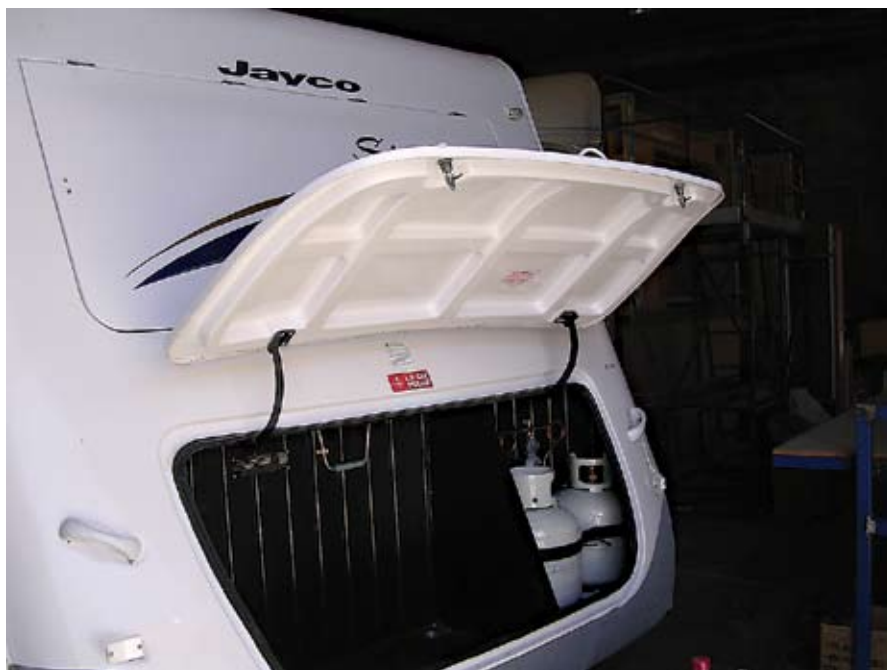
Caravan compartment (recess) constructed of material that is water and corrosion resistant
